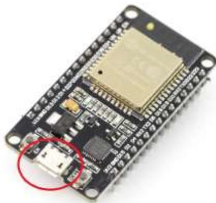
Fig. 2. Port for mini-USB cable on the ESP32 board.
